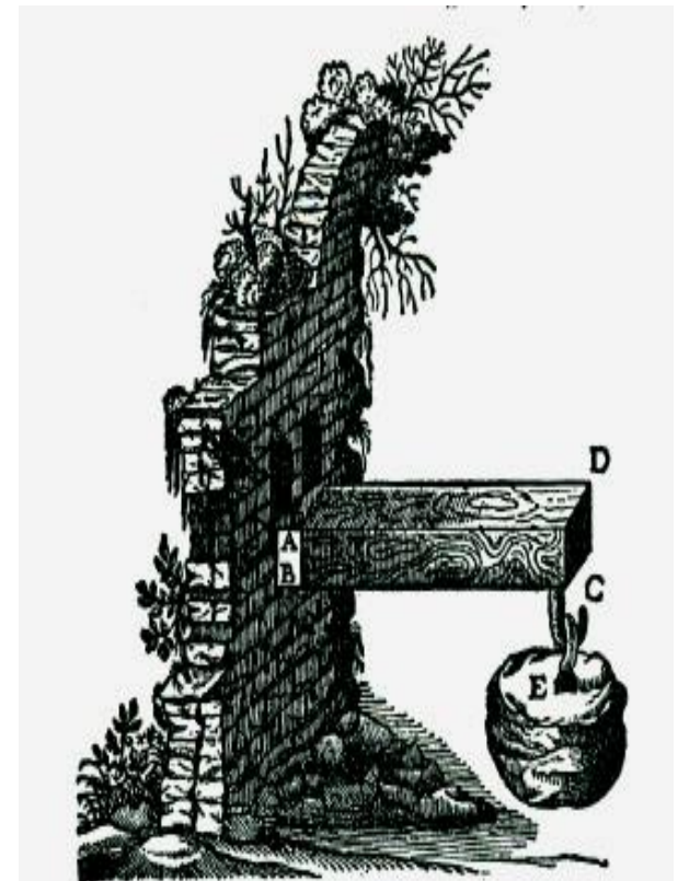
FIG. 15. Galileo's illustration of bending test.
