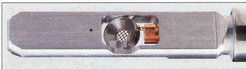
Tip of the Model 646 Double Tilt Analytical Holder, showing the ToggleTilt™ drive for the second tilt movement. Note the miniature Faraday cup and the cut-outs in the specimen cup and surrounding tip which minimize shadowing of the X-ray signal.
