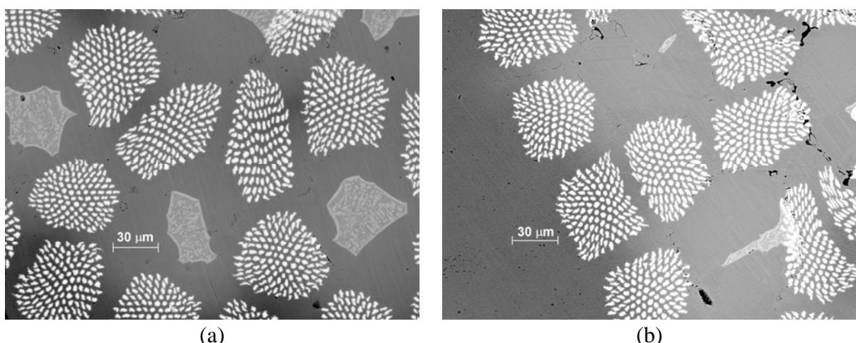
Fig. 3. Microstructures formed after heat treatments for: (a) Sample 3; (b) Sample 7. **Eutectoid decomposition of  $\gamma$  phase.**
