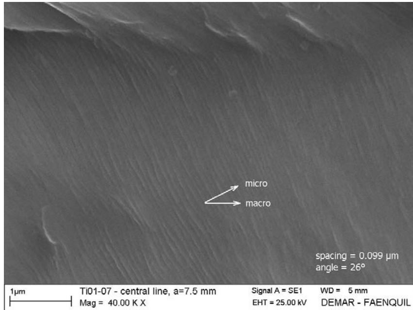
FIGURE 1 Representative SEM fractography of type A striation pattern (sample tested with  $R = 0.5$  and  $a = 7.5$  mm).
