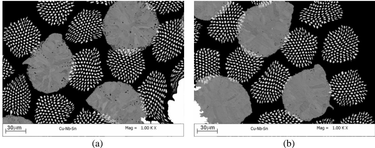
Fig. 1. Microstructures formed after heat treatments for: (a) Sample 1; (b) Sample 5. **Formation of  $\varepsilon$  phase.**
