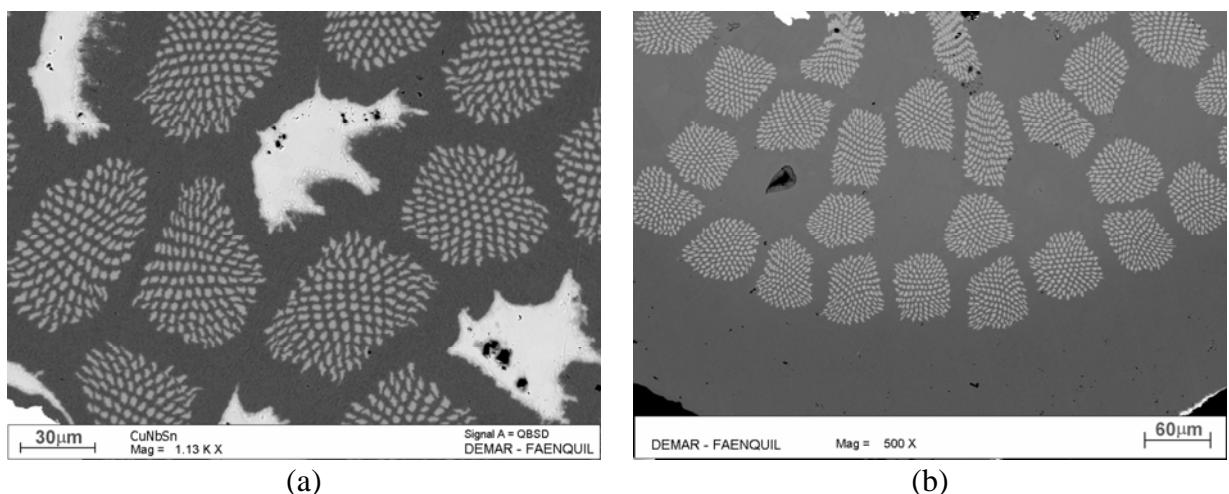
Fig. 4. Microstructures of sample 4 before (a) and after (b) heat treatment, showing the complete conversion of the Sn cores into  $\alpha$  phase.
