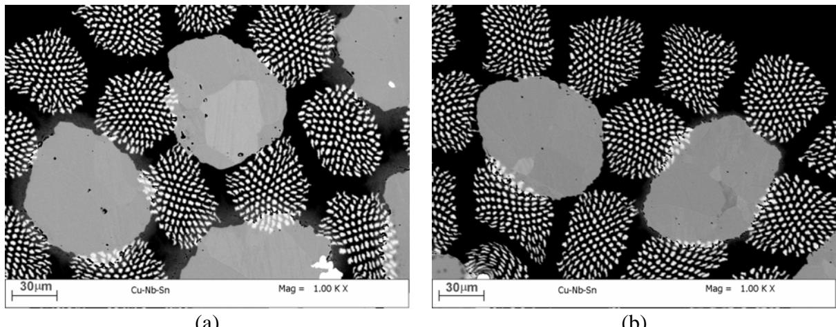
Fig. 2. Microstructures formed after heat treatments for: (a) Sample 2; (b) Sample 6. **Formation of  $\delta$  phase.**
