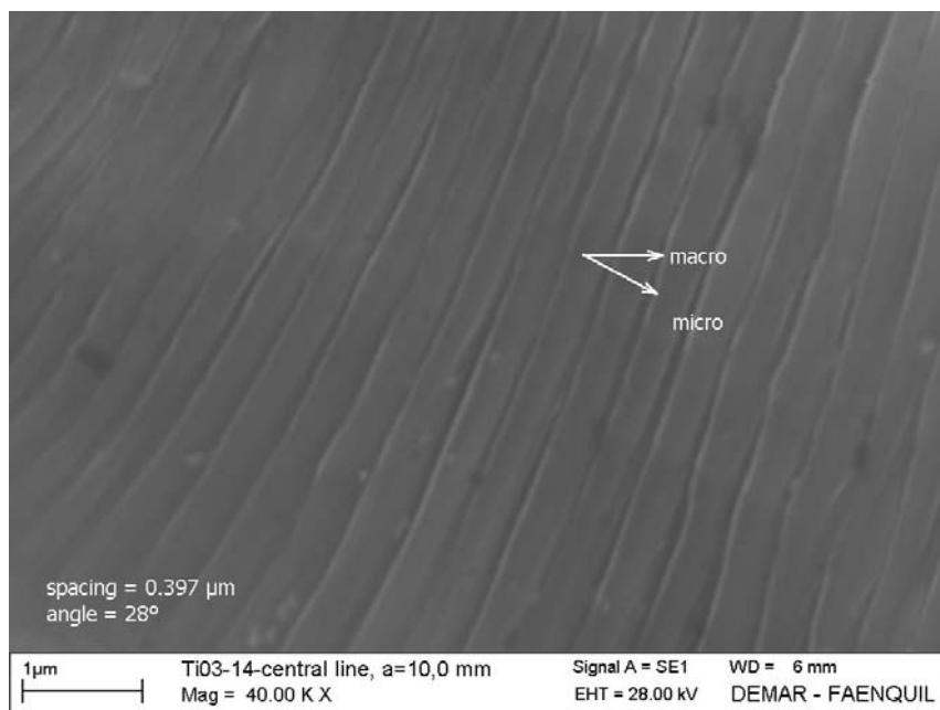
FIGURE 2 Representative SEM fractography of type B striation pattern (sample tested with  $R = 0.1$  and  $a = 10.0$  mm).
