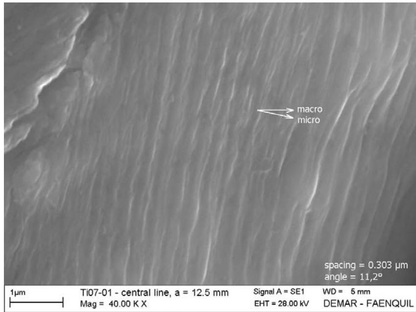
FIGURE 3 Representative SEM fractography of type C striation pattern (sample tested with  $R = 0.3$  and  $a = 12.5\text{ mm}$ ).
