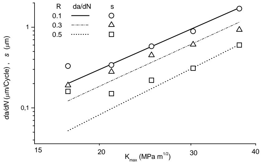
FIGURE 4 Fatigue crack growth rates and striation spacing.
