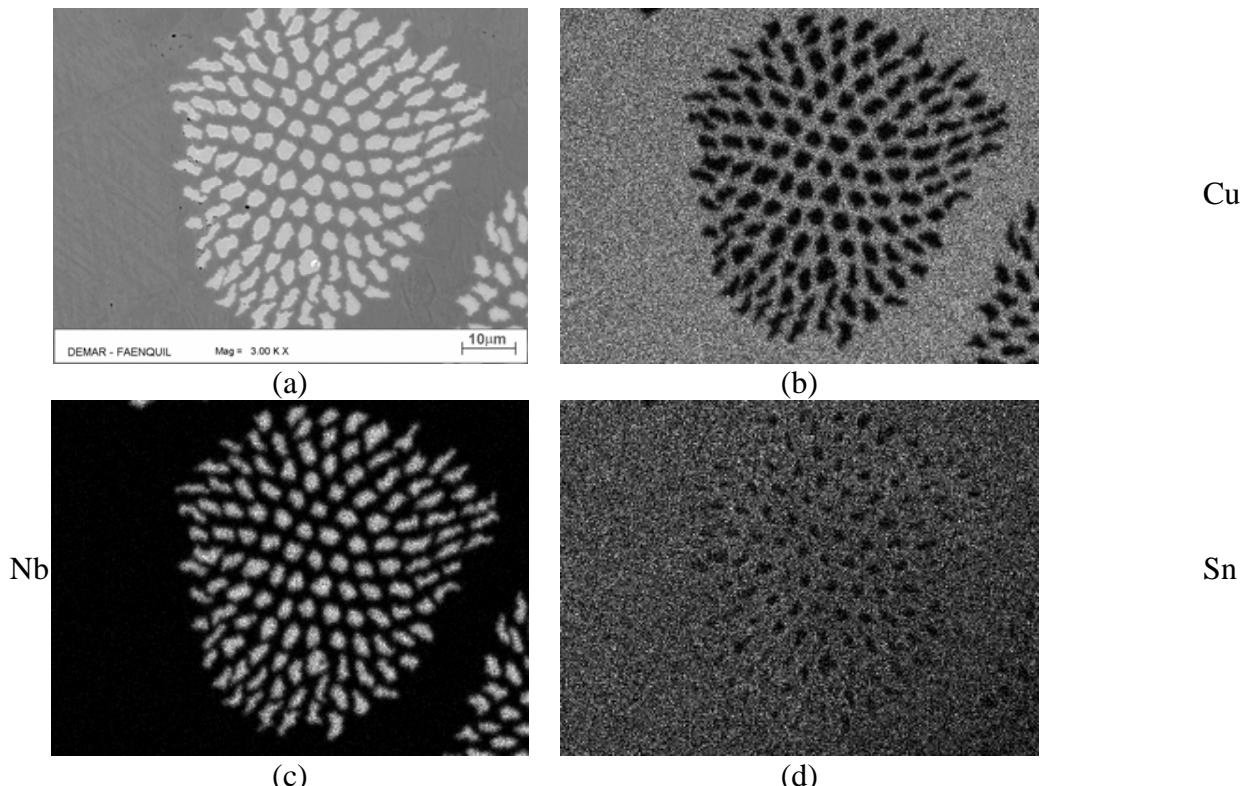
Fig. 6. Microstructure and X-ray mapping found using SEM+EDS for sample 4. (a) SEM image using backscattered electrons; (b) mapping of Cu; (c) mapping of Nb; (d) mapping of Sn. It can be noted the better homogenization of Sn compared to sample 2 (Fig. 5).
