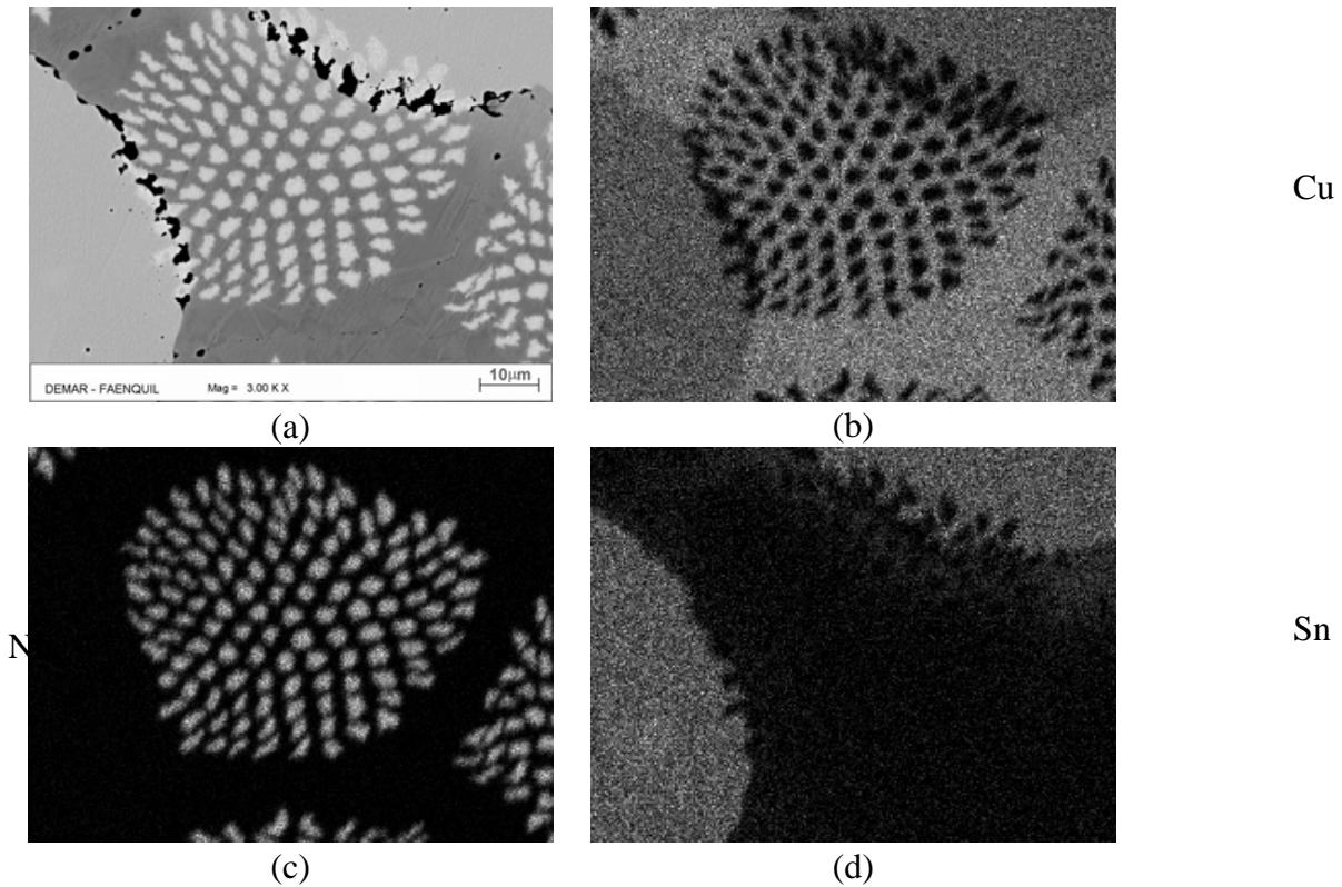
Fig. 5. Microstructure and X-ray mapping found using SEM+EDS for sample 2. (a) SEM image using backscattered electrons; (b) mapping of Cu; (c) mapping of Nb; (d) mapping of Sn.
