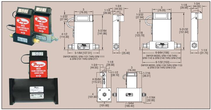
Series GFM Gas Mass Flow Meters combine a straight tube sensor with a restrictor flow element to provide high accuracy and repeatability. Flow rates are virtually unaffected by temperature and pressure variations. Actual gas flow is displayed in engineering units on a 3-digit, 90° tiltable LCD readout. Units can be used with Series GFT Flow Totalizer for applications requiring totalization. Series GFM includes a NIST traceable certificate.
