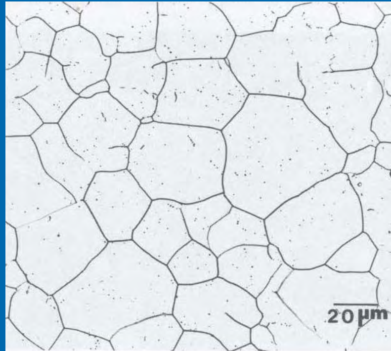
Fig. 8.46 Annealed AISI/SAE 316 austenitic stainless steel showing grain boundaries but the absence of twins. Ideal for grain size measurements by image analysis. Electrolytically etched with 60% nitric acid and 40% water using a platinum cathode at 5 V. 500×
