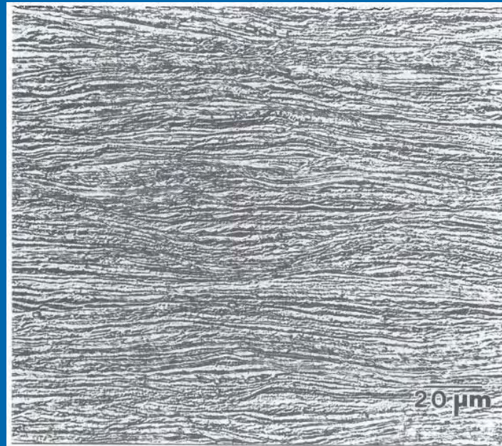
Fig. 8.45 Heavily cold-worked AISI/SAE 301 austenitic stainless steel. Electrolytically etched in 10% oxalic acid solution using a stainless steel cathode at 8 V. Enhanced by differential interference contrast illumination (also called Nomarski illumination). 500×
