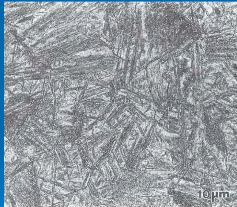
Fig. 2.34 Lower bainite in an AISI/SAE 8720 steel isothermally transformed at 325 °C (617 °F) for 100 s. 4% picral etch. 800×
