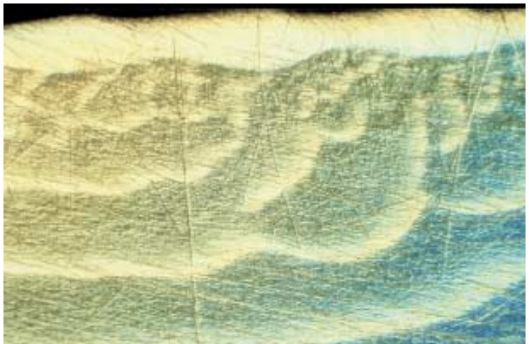
2. Smearing on soft, ductile steel Mag: 25 x, DIC
