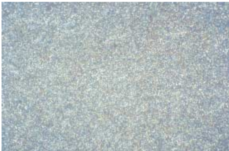
100 Cr 6 Mag: 500x Etchant: Nital
