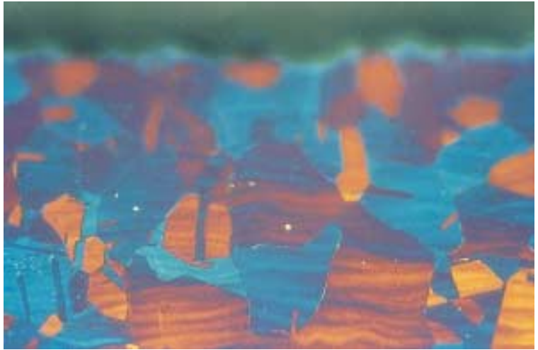
1. Due to a gap between resin and sample the edge is rounded. Stainless steel. Mag: 500 x Etchant: Beraha I
