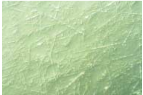
2. Well-defined, sharp deformation lines Mag: 200 x, DIC
