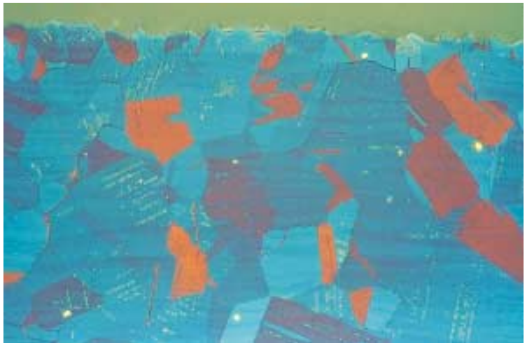
2. Good edge retention, stainless steel Mag: 500 x Etchant: Beraha I
