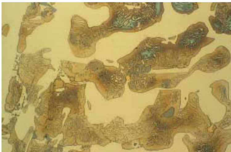
White cast iron Mag: 500x Etchant: Klemm I
