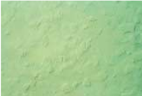
1. Short deformation lines, restricted to single grains. Mag: 100 x, DIC
