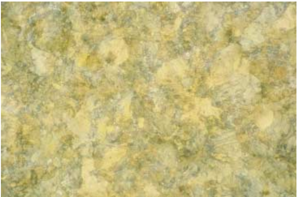
Tool steel Mag: 200x Etchant: Nital
