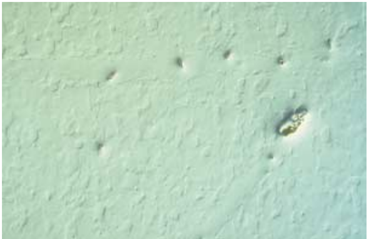
2. Lapping tracks after final polishing. The very deep indenta- tions can still be seen. Also visible is the under- lying deformation following the lap- ping track. Pure Tantalum Mag: 500 x, DIC
