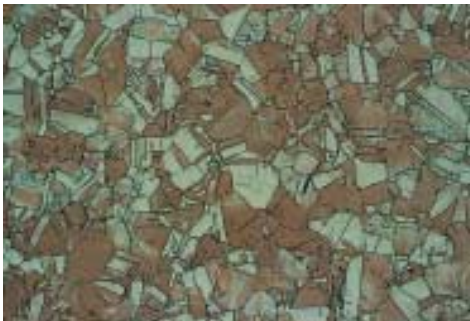
Copper pure Mag: 50x Etchant: Copper ammonium chloride
