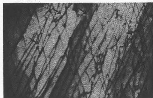
Fig. 27, 28, 29 Oriented dislocation arrays in thin foils. Fig. 27: copper. (Ref 15). Fig. 28: iron. (Ref 15). Fig. 29: Armco iron. (Ref 18). Etchants and magnifications not reported
