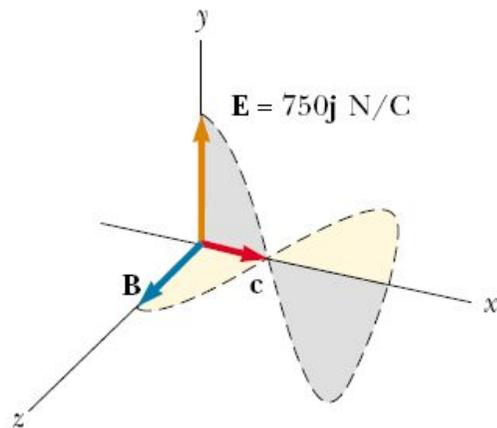
**Figure 34.4** At some instant, a plane electromagnetic wave moving in the  $x$  direction has a maximum electric field of 750 N/C in the positive  $y$  direction. The corresponding magnetic field at that point has a magnitude  $E/c$  and is in the  $z$  direction.
