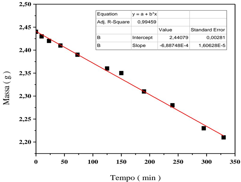
$$W'_{A,r} = -(-6,89 \times 10^{-4}) \text{ g/min} = \frac{6,89 \times 10^{-4} \text{ g/min}}{60 \text{ s/min}}$$
