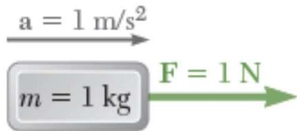
$$1 \text{ N} = (1 \text{ kg}) (1 \text{ m/s}^2) = 1 \text{ kg} \cdot \text{m/s}^2$$
