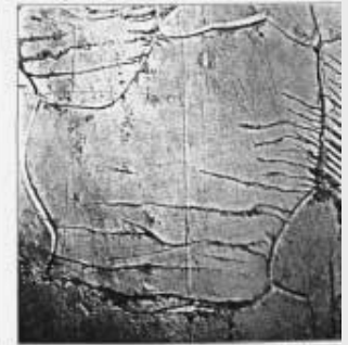
Fig. 12. Specimen after 40,000 reversals. \times 1000 .
