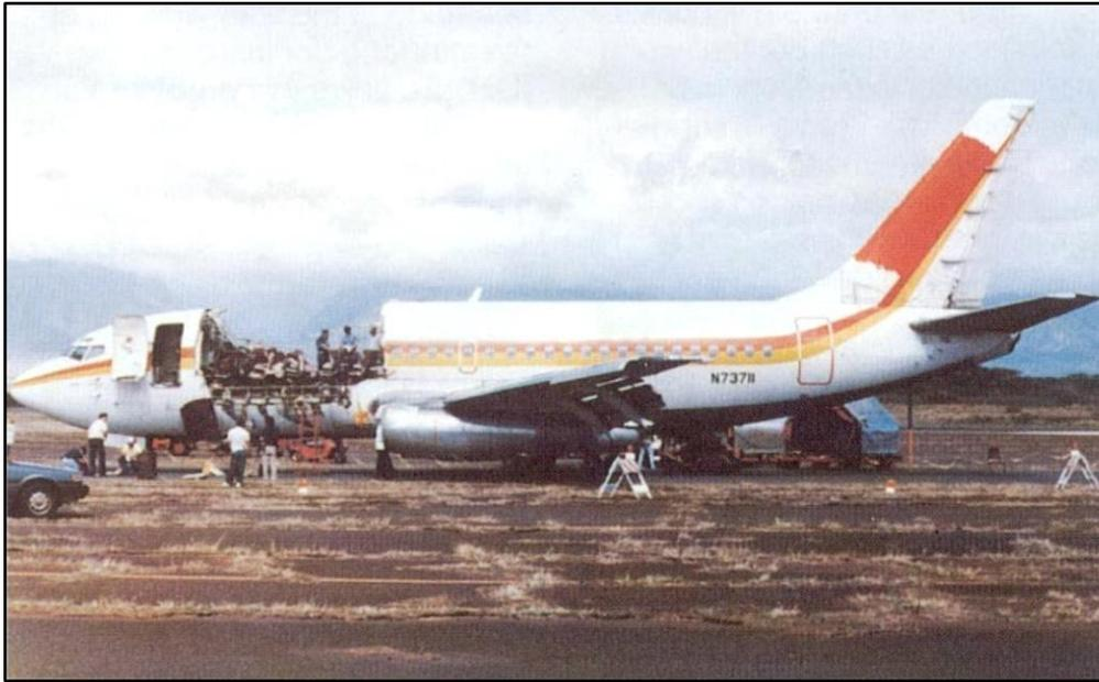
At the time of the accident, the N73711 had accumulated 35,496 flight hours and 89,680 flight cycles (landings), the second highest number of cycles in the worldwide B-737 fleet. Due to the short distance between destinations on some Aloha Airlines routes, the maximum pressure differential of 7.5 psi was not reached on every flight. Therefore, the number of equivalent full pressurization cycles on the accident airplane is significantly less than the 89,680 cycles accumulated on the airplane.
