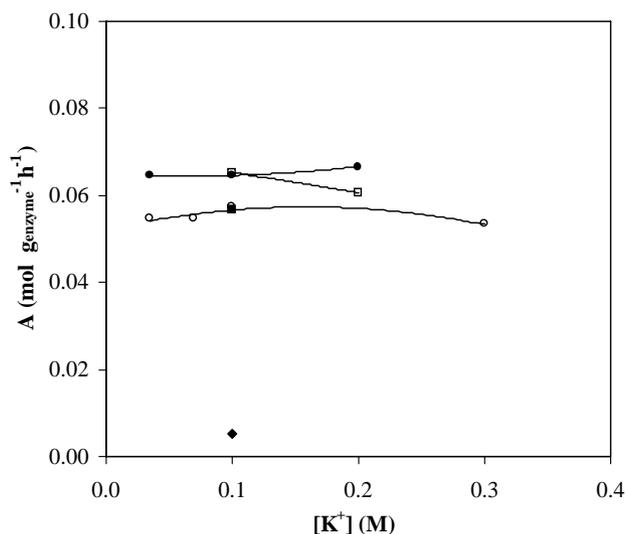
Fig. 1. Influence of pH and  $[K^+]$  on the activity of Lactozym. Citric-phosphate buffer,  $[PO_4^{3-}] = 0.01$  M, fit of  $[K^+]$  by KCl addition,  $[Mg^{2+}] = 0$  M. (◆) pH 6.00, (○) pH 6.50, (●) pH 6.75, (□) pH 7.00 and (■) pH 7.30.
