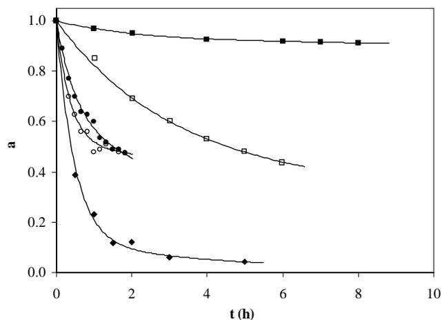
Fig. 8. Fit of the proposed deactivation model to the experimental data obtained by different authors [16] (soluble enzyme): (■) 40°C, (□) 45°C, (◆) 50°C [26], (●) 45°C, soluble enzyme, (○) 45°C, immobilized enzyme.
