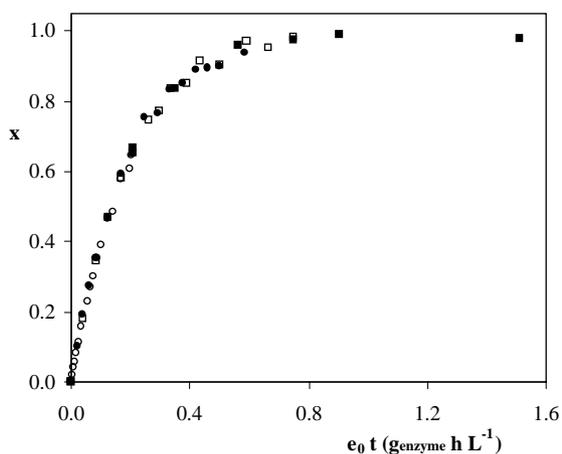
Fig. 9. Influence of lactose concentration on Lactozym activity. Buffer  $\text{K}^+$  and  $\text{Mg}^{2+}$ . Lactose concentration =  $25 \text{ g l}^{-1}$ , 40°C.  $e_0$ : (○)  $0.1 \text{ g l}^{-1}$ , (●)  $0.5 \text{ g l}^{-1}$ , (□)  $1.0 \text{ g l}^{-1}$ , (■)  $3.0 \text{ g l}^{-1}$ .
