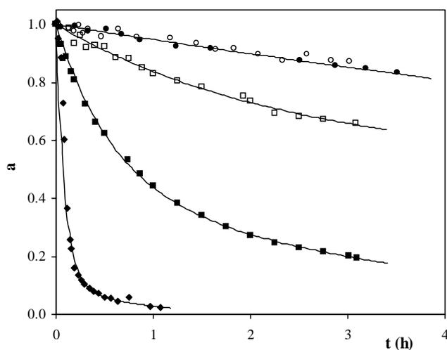
Fig. 4. Fit of the proposed model to the relative activity vs. temperature. Buffer  $K^+$  and  $Mg^{2+}$ . Lactozym: (○) 40 °C, (□) 42.5 °C, (■) 45 °C, (◆) 50 °C and Maxilact: (●) 40 °C. (—) Model proposed.
