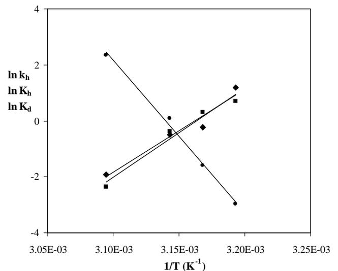
Fig. 6. Temperature dependence of  $k_h$ ,  $K_h$  and  $K_d$ . Buffer  $\text{K}^+$  and  $\text{Mg}^{2+}$ . Lactozym and Maxilact. (●)  $k_h$ , (■)  $K_h$ , (◆)  $K_d$ .
