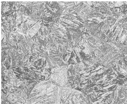
Fig. 15.11 Lath martensite. Source: Ref 15.4 as published in Ref 15.2
