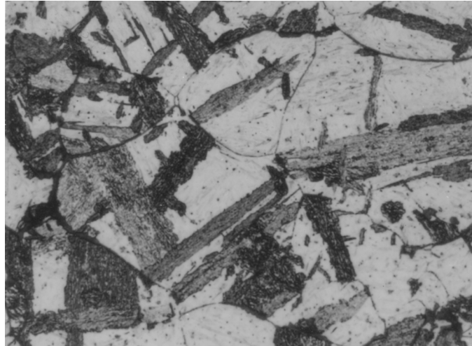
Fig. 15.31 Upper bainite (dark rectangular areas) in 4150 steel transformed at 460 °C (860 °F). Original magnification: 500 \times . Courtesy of Florence Jacobs, Colorado School of Mines. Source: Ref 15.19
