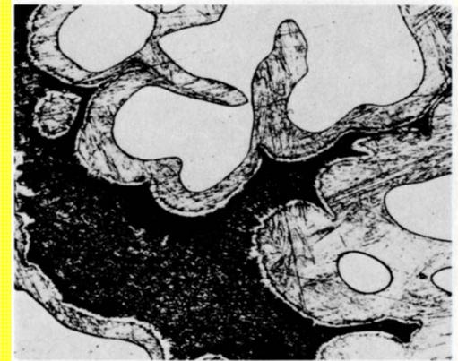
**Fig. 9** Start of the peritectic transformation in the same directionally solidified Cu-20Sn alloy shown in Fig. 7, but at higher magnification. Note the homogeneous thickness of the β layers (gray) around the primary α (white). The matrix (dark) is a mixture of tin-rich phases. Mechanically polished, etched in HNO<sub>3</sub>. 160×. (Ref 6)
