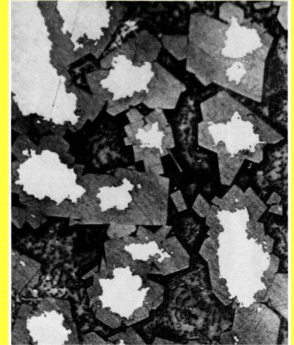
**Fig. 18** Peritectic envelope in a Bi-40Au alloy that was cooled to 450 °C (840 °F) and held 5 h, then cooled to 300 °C (570 °F) and held 2 h (peritectic temperature: 373 °C, or 703 °F). The morphology is entirely determined by the anisotropy of the interfacial energy of the face-centered cubic  $Au_2Bi$  crystals (gray). The primary crystals are gold (white); the matrix is the  $Au_2Bi$ -Bi eutectic. Mechanically polished, contrasted by reactively sputtered interference layer. 200×
