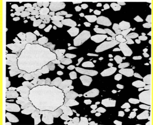
**Fig. 15** Microstructure of a Cd-10Cu alloy that was cooled to 410 °C (770 °F) and held 20 h, then cooled to 305 °C (580 °F) and held 160 min (peritectic temperature: 397 °C, or 747 °F). Note the faceted coarse crystals of the peritectically formed CuCd<sub>3</sub> envelopes (gray). The primary Cu<sub>5</sub>Cd<sub>8</sub> crystals are white; the dark matrix is cadmium. Mechanically polished, etched in HNO<sub>3</sub>. 100×
