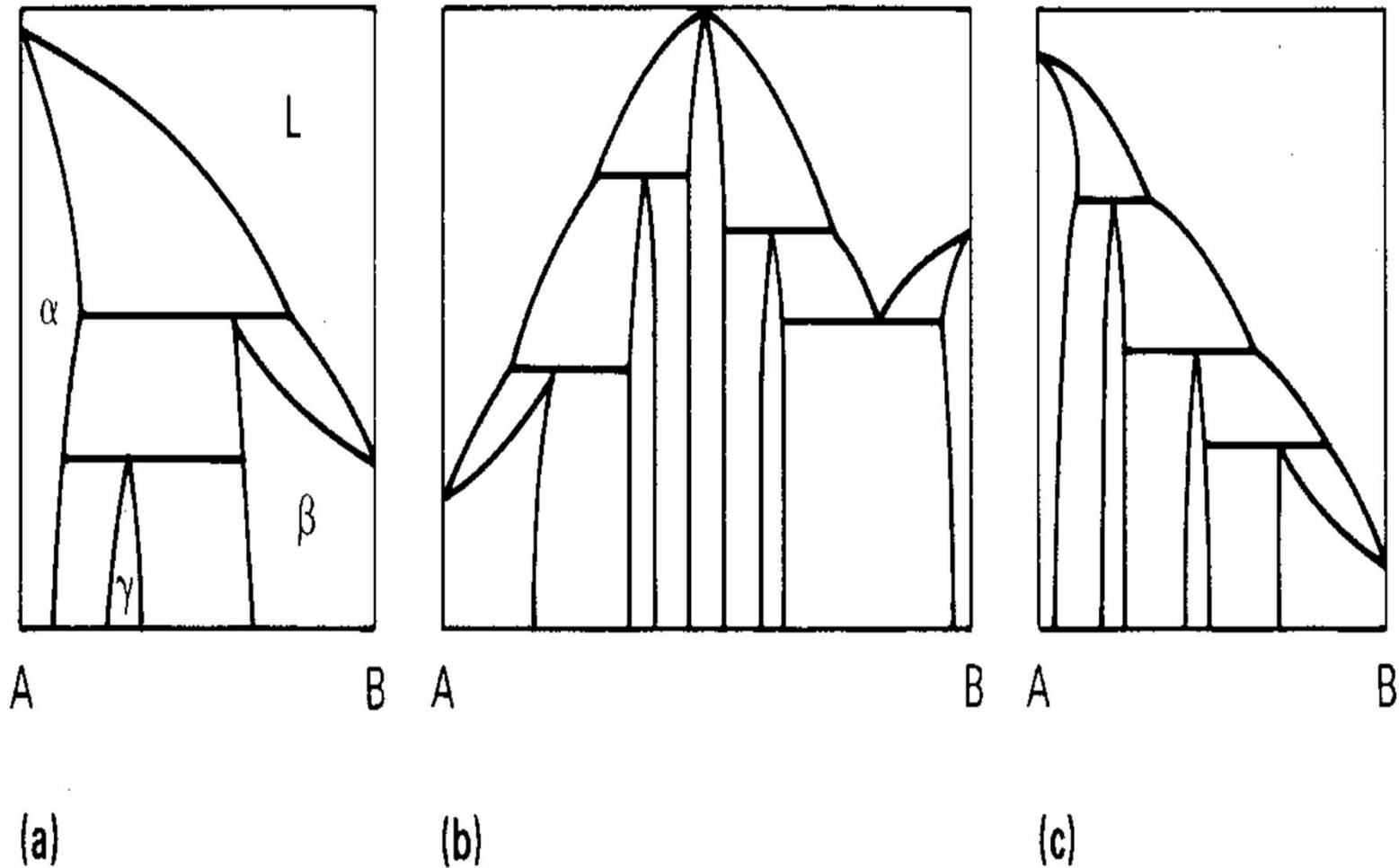
**Fig. 1** Typical peritectic phase diagrams. (a) Peritectic reaction  $\alpha + \text{liquid} \rightarrow \beta$  and peritectoid reaction  $\alpha + \beta \rightarrow \gamma$ . (b) Peritectic formation of intermetallic phases from a high-melting intermetallic. (c) Peritectic cascade between high- and low-melting components.
