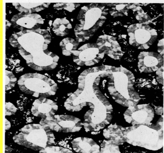
**Fig. 16** Same as Fig. 15, except alloy was cooled to 410 °C (770 °F) and held 20 h, then cooled to 275 °C (525 °F) and held 160 min (peritectic temperature: 397 °C, or 747 °F; eutectic temperature: 314 °C, or 597 °F). Note large number of grain boundaries in the peritectic CuCd<sub>3</sub> phase (gray) and its smooth interfaces with the primary Cu<sub>5</sub>Cd<sub>8</sub> crystals (white) and the matrix Cd (dark). 100×
