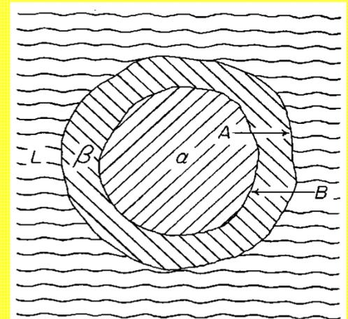
**FIG. 8-4.** Schematic representation of primary α undergoing peritectic reaction with liquid L to form an envelope of β. The reaction progresses by the diffusion of A atoms outward and B atoms inward through the shell of β.
