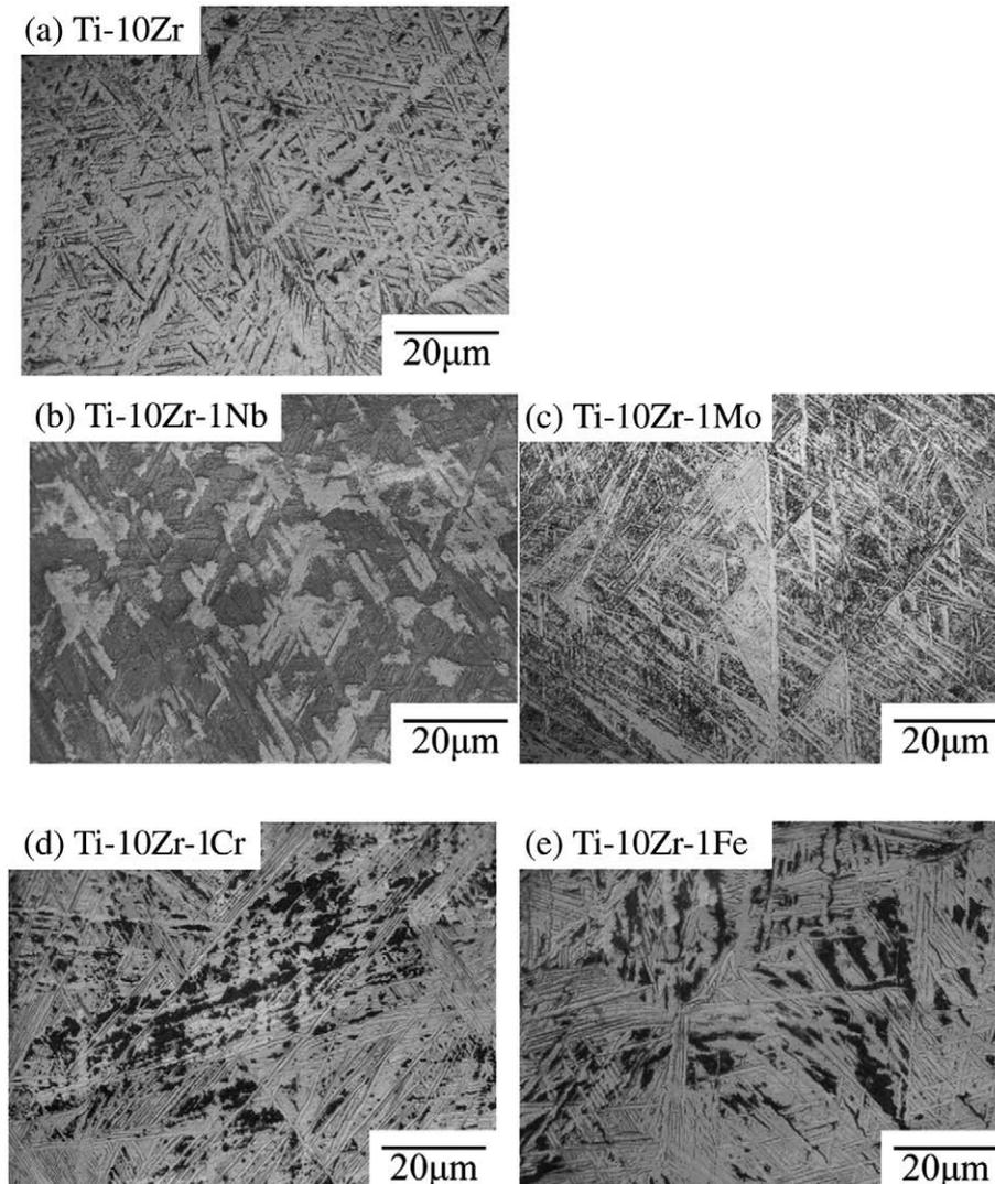
Fig. 1. Light micrographs of Ti–10Zr and Ti–10Zr–1X alloys.
