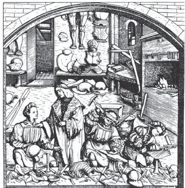
Fig. 15. Armourer's workshop of the XVI century A.D. Showing some of its products and the tools used in making them [7,15].
