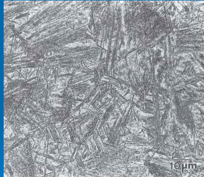
Fig. 2.34 Lower bainite in an AISI/SAE 8720 steel isothermally transformed at 325 °C (617 °F) for 100 s. 4% picral etch. 800X
