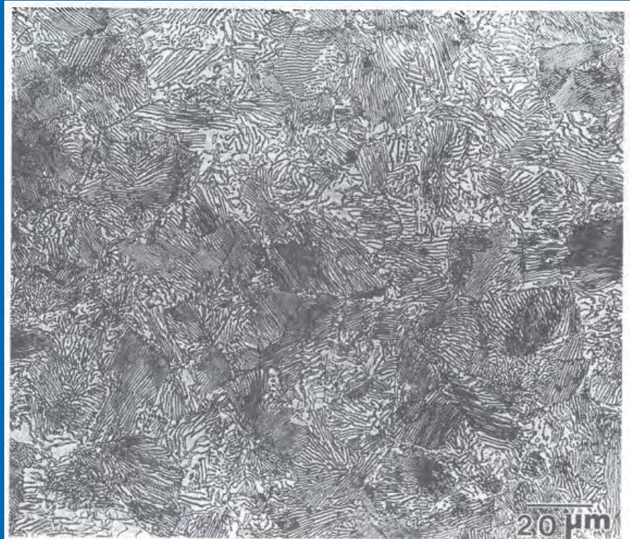
Fig. 1.2(c) Micrograph of high-carbon AISI/SAE 1095 steel showing a matrix of pearlite and some grain-boundary cementite. Etched in 4% picral. 500X
