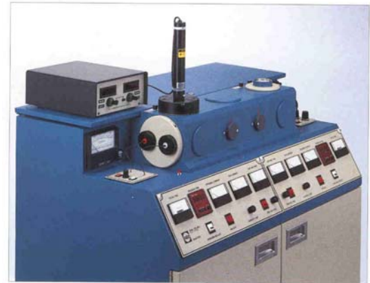
The Laser Autoterminator Control Unit operates with one or two Laser Head assemblies (which seat over the airlock capsule) to provide automatic termination of milling.
