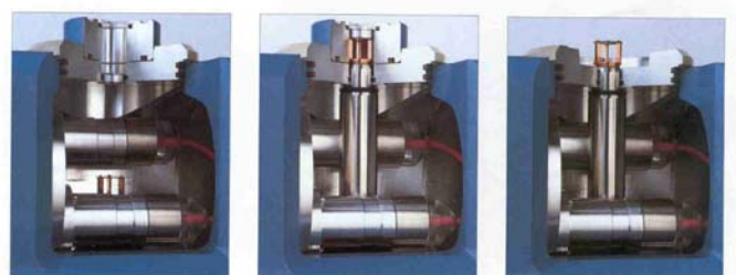
Close-up views of a cut away DuoMill™ illustrate the operation of the Whisperlok™. In the lower, working position (left) the sputter shield prevents material from the specimen coating the airlock capsule window. Simply by pressing the "Raise" switch the specimen holder is gently moved up into the airlock (center). Once in position, the "Air" button is pressed to admit air to the airlock capsule which can then be removed (right).
