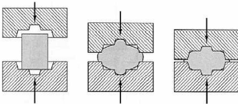
Schematics of the impression-die forging process showing partial die filling at the beginning of flash formation in the center sketch, and the final shape with flash in the right-hand sketch
