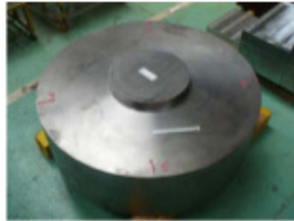
Figure 24 12Cr steel disc for welding test with LTES700R (Courtesy of Mitsubishi Heavy Industries)
