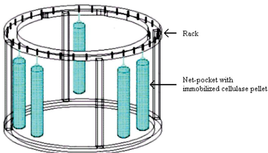
Fig. 1. (A) The schematic diagram of the hanging immobilized cellulase reactor. (B) The net-pocket filled with the immobilized cellulase pellets and hung under the rack.
