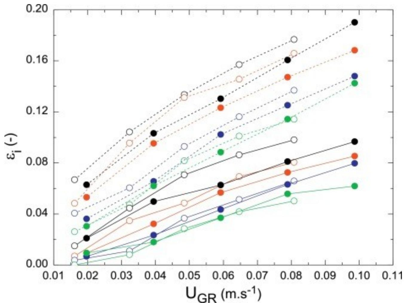
Fig. 2. Typical behavior of the gas hold-up in the riser and downcomer ( $\varepsilon_i$ ) as a function of superficial gas velocity in the riser ( $U_{GR}$ ), found for Newtonian and non-Newtonian fluids in DTA and SCA reactors. The plotted data refers to the CMC solutions in SCA reactor. Legend: (●) CMC15-5L, (○) CMC25-5L, (○) CMC35-5L, (○) CMC45-5L, (●) CMC15-10L, (●) CMC25-10L, (●) CMC35-10L, (●) CMC45-10L; (---)  $\varepsilon_R$ , (—)  $\varepsilon_D$ .
