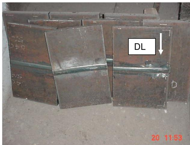
Figura 3.12 - Amostras-3: chapas soldadas (SAW).
